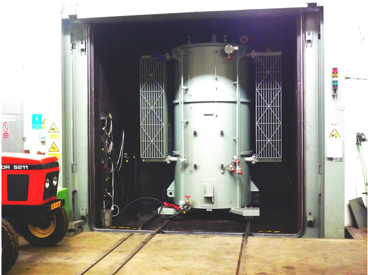
Vacuum drying chamber for drying arc suppression coils
