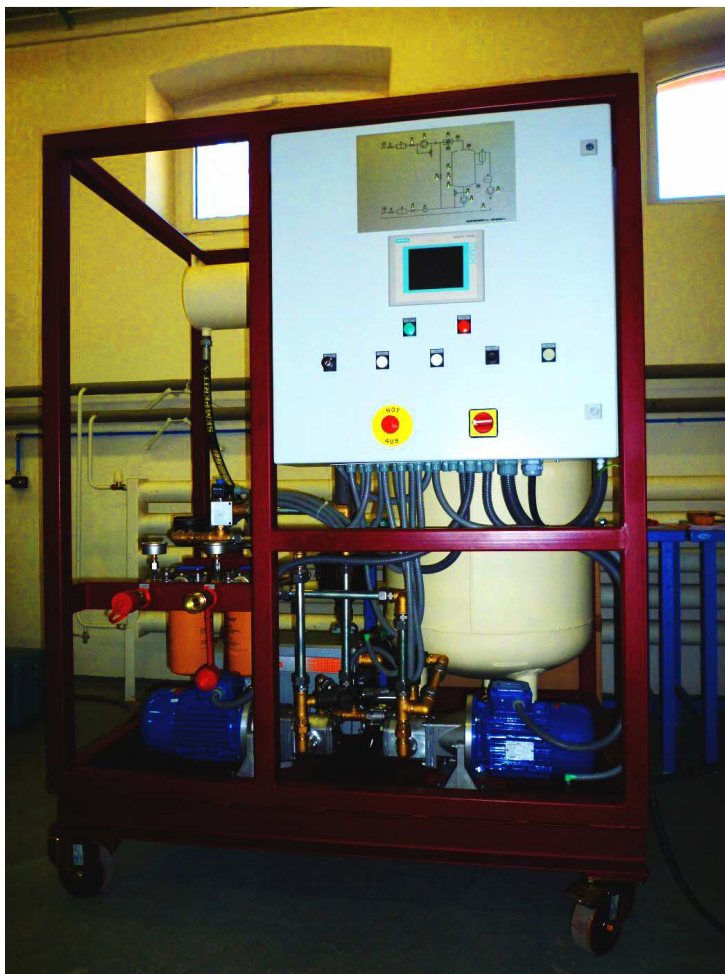
The filtration unit TPF500 – 500 l/hr
